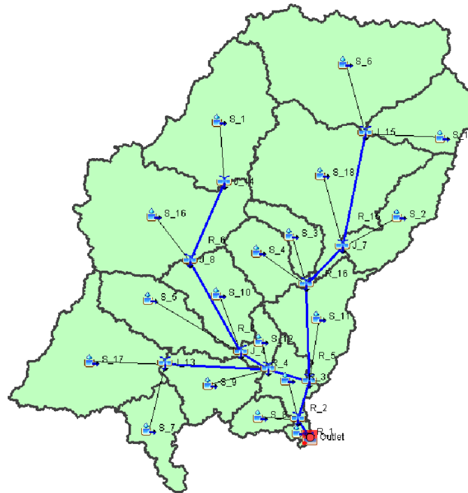
Figure 7. Schematic representation of zone-12 watershed delineated from CartoDEM using HEC-HMS 4.6 version.
