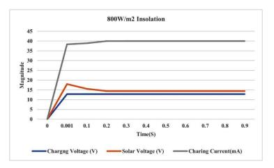
Figure 9. Lab performance of solar charger using soft computing technique under 800W/m2 insolation.
