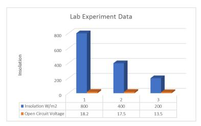
Figure 8. Solar panel open circuit voltage under various conditions of insolation.
