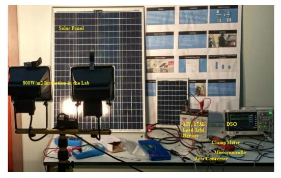
Figure 4. A hardware model for solar battery charger using soft computing techniques.
