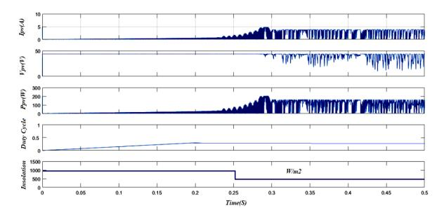
Figure 6. An incremental conductance based algorithm performance under 1000w/m2 and 500w/m2 of insolation.
