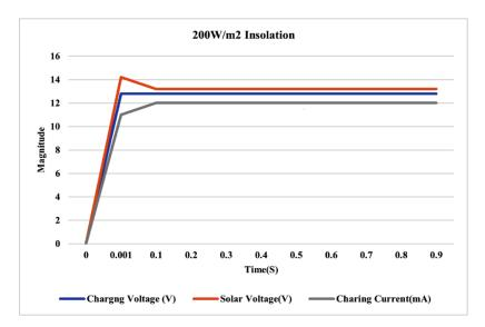
Figure 11. Lab performance of solar charger using soft computing technique under 200W/m2 insolation.
