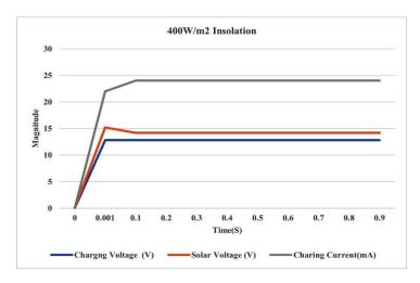
Figure 10. Lab performance of solar charger using soft computing technique under 400W/m2 insolation.
