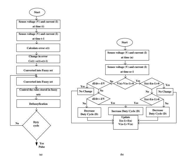
**Figure 3.** (a)-(b) Soft computing intelligent algorithm for generation pulse at MPPT and an incremental conductance algorithm to generate pulse at MPPT.
