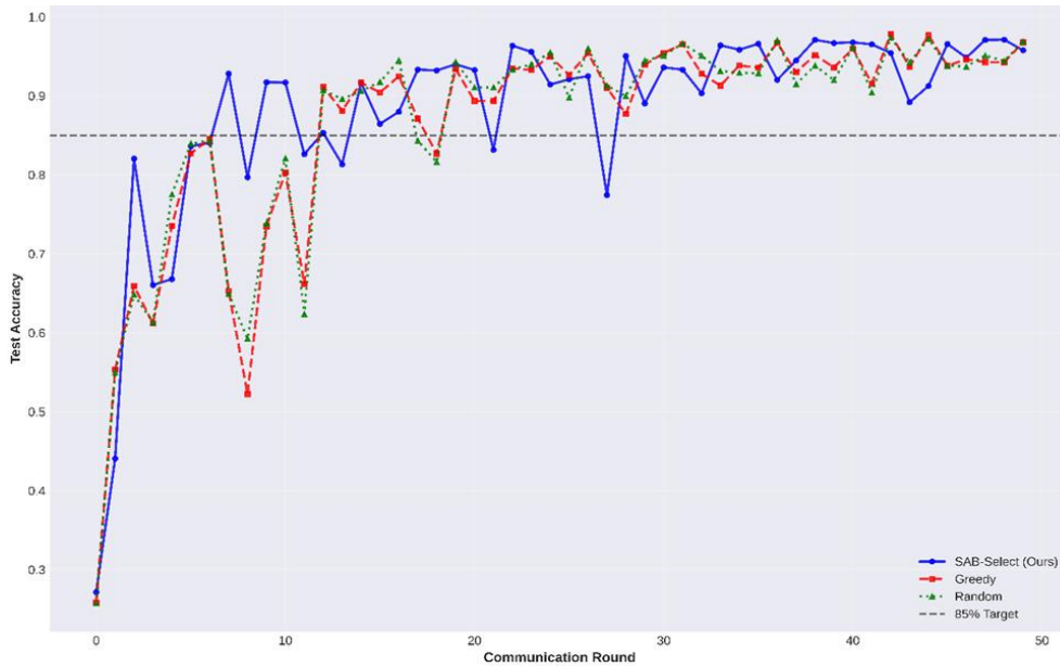
Figure 3. SAB-Select achieves 85% target accuracy in 7 rounds 2x faster than baselines under bursty connectivity.
