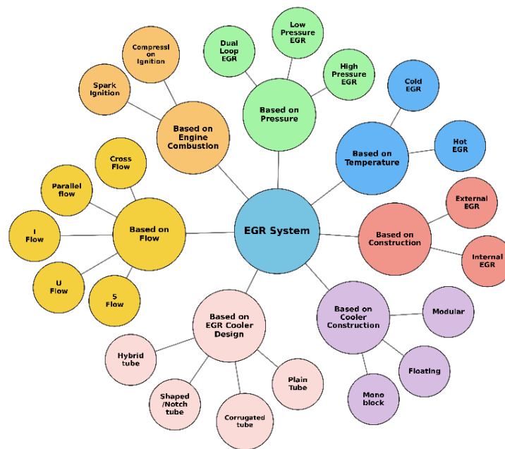
Figure 3. Mind map of the EGR system classification by design, application, and location.
