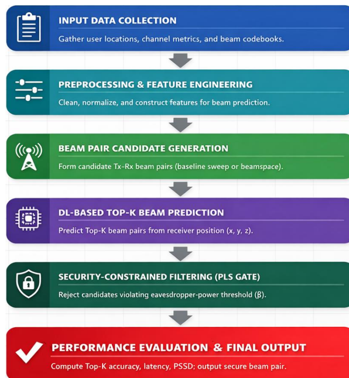
Figure 2. Beam selection and alignment process in 5G.
